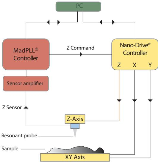
The configuration described above is a highly flexible 3 axis closed loop AFM. The **SPM-M kit** is a pre-configured package for a 3 axis closed loop AFM that is quick to assemble and easy to upgrade with our wide range of accessories.
