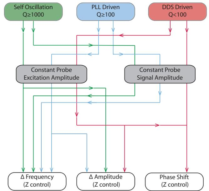
*The digital MadPLL® controller has three operational modes: self oscillation, PLL driven, and DDS driven. The probe can be controlled in constant excitation amplitude or constant signal amplitude. Changes in frequency, amplitude, or phase are measured for Z control.*
