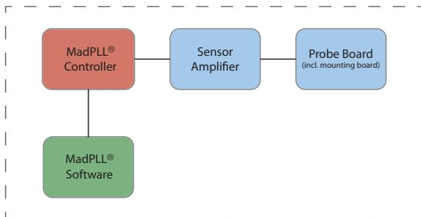
*The MadPLL® package includes the MadPLL® digital PLL controller, sensor amplifier, probe board and MadPLL® software. Ease of integration with resonant probes and Mad City Labs’ low noise, closed loop nanopositioning systems give users the ability to create high performance, low cost NSOM and AFM instruments.*
