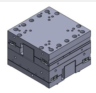
4 x C-Bored for M3 SHCAP screws on a 72mm x 42 mm rectangle
