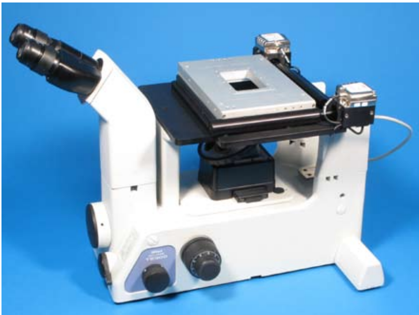
Nano-View® 300-3 (2-axis (XY) micropositioning plus 3-axis (XYZ) nanopositioning) mounted on a Nikon inverted microscope.
