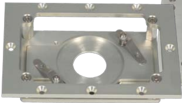
Re-entrant slide holder with coverslip adapter.
