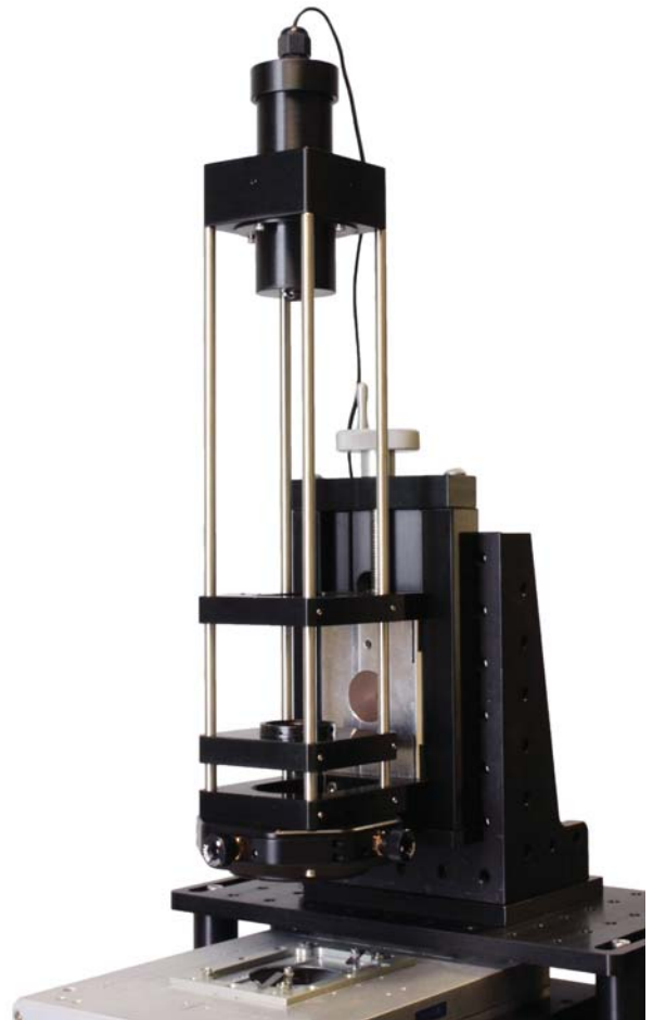
Köhler illumination tower on a RM21™ microscope with Nano-LPS nanopositioner.
